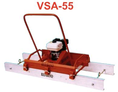
The **Red Band VSA-55** Vibrating Screeder drive unit is strongly built from jig welded steel for use in the toughest of site conditions, enabling concrete to be laid efficiently and with less effort than conventional methods; now with increased vibration for enhanced consolidation. The unit is designed so that maximum vibration is concentrated on the leading beam, with lighter vibration applied to the following beam to achieve a smooth finish.
