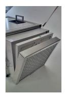
The H13/14 hepafilter can be replaced by following the same procedure as above. If you use the machine daily we would recommend changing the hepafilter once a year. Of course, this depends on the contaimination of the air in the environment. At the top of the hepafilter you will find a label with the item number (compare this number with the number on the old filter). Make sure you place the filter as indicated on the label: **^Airflow**.
