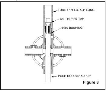
2. Using the opposite end or short end of installation tool #06703, install (4) outer bushings into spider.
