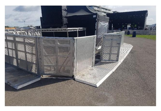
Image showing a 1m front of stage stage/pedestrian gate being used to create access to the front of house area the front of house area has been barrierd all the way round so the gate is the only access creating a secure area.
