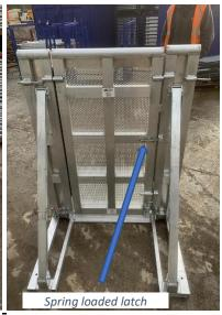
1m Front of stage, stage/pedestrian gate in the closed position showing how the gate continues the streamline continuation of the line of front of stage barriers
