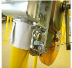
**Illustration 3** press ball pin to hold winch in place.
