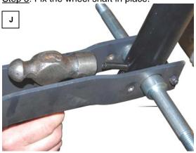
Rotate the wheel shaft until the hole for the retaining pin aligns with the opening in steering the shaft; then tap the retaining pin into place. K. Reinstall the cross-link and tighten fasteners.
