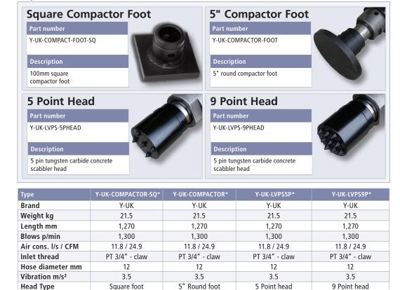
\*Supplied as a complete unit with compactor and detailed head type
