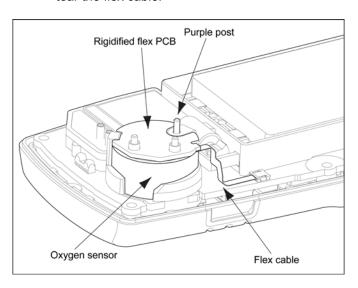
Note the placement of the PCB to ensure it is replaced correctly. Remove the two screws on the PCB.
