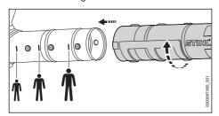
► Adjust blower tube to the desired position.
