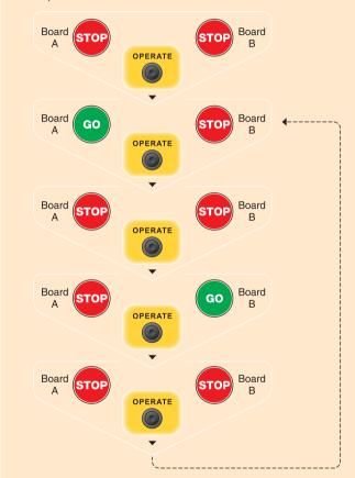
For added safety there is a four second delay after every change of state before the next step of the sequence can be activated. During the four second period, a further press of the remote control **OPERATE** button will have no effect.
