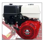
The engine is fitted with a fuel on/off lever and a choke lever. Read the engine operating instructions to understand the operation of these levers.
